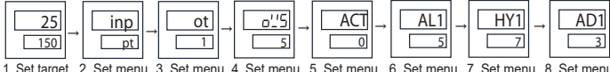
1. Set target temperature SV=150 2. Set menu INP=pt 3. Set menu OT=1 4. Set menu OVS=5 5. Set menu ACT=0 6. Set menu AL1=5 7. Set menu HY1=7 8. Set menu AD1=3
